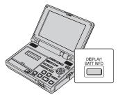
After a while, the approximate available playback time and battery information appear for about 7 seconds. You can view the battery information for up to 20 seconds by pressing DISPLAY/BATT INFO again, while the information is displayed.
